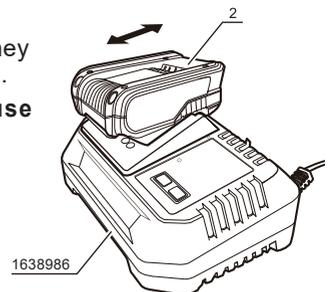
1. Plug the battery charger into the proper AC voltage source. A steady GREEN light will illuminate indicating the charger is connected to a proper power source.
