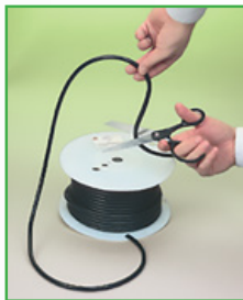
Cut rope one-third shorter than the finished length
