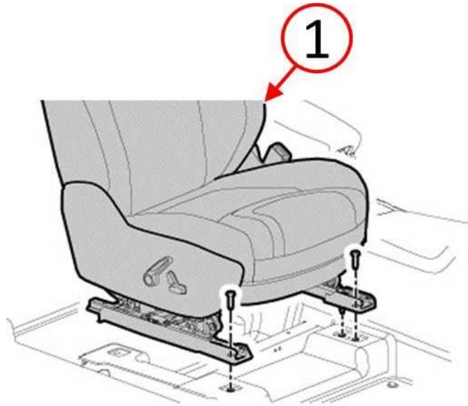
Fig. 2 Remove Right Side Front Seat
