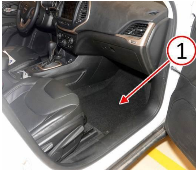
Fig. 1 Water In Right Side Front Footwell
