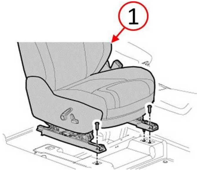
Fig. 19 Install Right Side Front Seat
