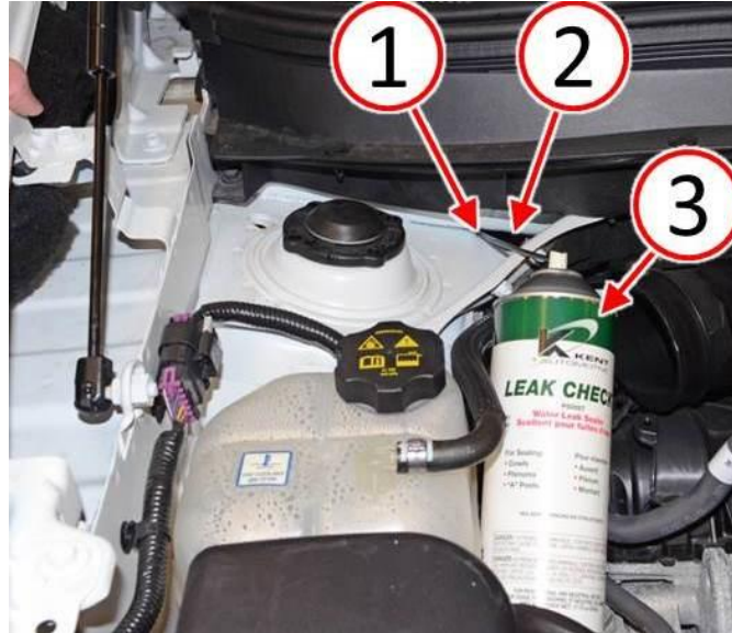
Fig. 10 Apply Seam Sealant
