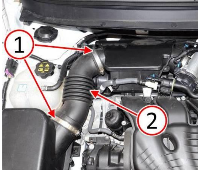
Fig. 8 Remove Engine Air Inlet Duct
