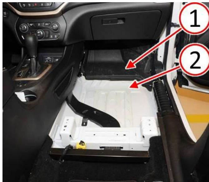
Fig. 12 Inspect For Water Leak
