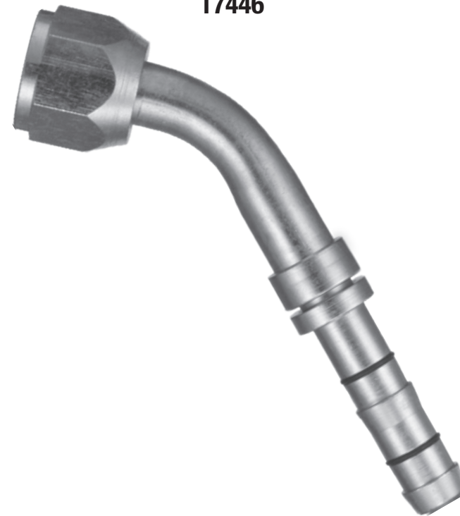
13/32 (-8) x 3/4-16 (-8) 45° Elbow Female O-Ring Short Pilot
