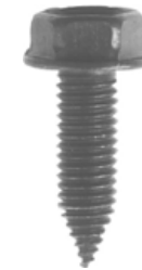
M8 x 1.25 x 25mm Hex Washer Head Body Bolt
