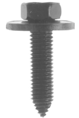
M10 x 1.5 x 40mm Hex Head Body Bolt with 28mm Captive Washer
