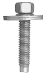
M6 x 1.0 x 25mm Hex Head Body Bolt with 19mm Captive Washer, 8mm Hex
