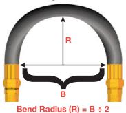
When determining the proper length of hose, it is important to make sure that the minimum bend radius is not exceeded. If the bend radius is smaller than the minimum, the hose could kink and burst. For example, if a hose has a minimum bend radius of 6", anything less than 6" would exceed this.
