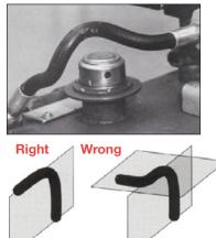
Proper fitting selection and orientation is an important part of hose routing. Using two rigid fittings on a hose will cause the hose to twist during installation. If a rigid fitting is used on one end of the hose, that end should be the first end installed. The other end should have a swivel fitting. This will enable the hose to stay straight without twisting. A hose twisted as little as 7° can have a 90% reduction in service life.
