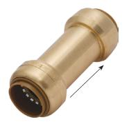
The Cash Acme SharkBite® Check Valve is a general-purpose spring check valve that prevents the reverse flow of water. It can be installed horizontally or vertically and can be connected in seconds to copper tubing, CTS, CPVC and PEX. The information below is specific to the SharkBite® Check Valves
