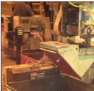
Thread-rolling machine dropping screws into hopper
