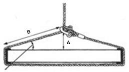
When this angle is less than  $45^{\circ}$ , SWL = SWL (of single vertical hitch) × A/B
