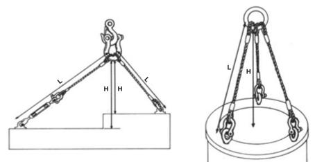
When sling legs are not of equal length, use smallest H/L ratio.
