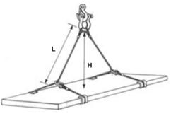
SWL = SWL (for vertical hitch)  $\times$  A/B  $\times$  H/L  $\times$  2
