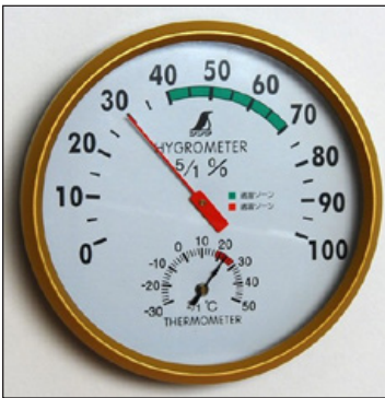
Hygrometer A gauge used for measuring atmospheric humidity
