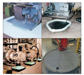
The style of the sorbent used is determined by the application.
