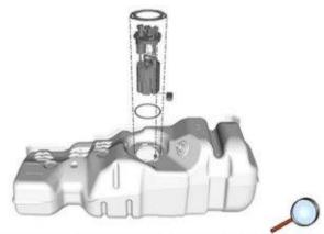
Remove the fuel tank fuel pump module. Refer to Fuel Tank Fuel Pump Module Replacement in ST.
