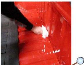
Use a rag and wax/grease removing solvent such as Acrysol, or equivalent, to remove any dirt, grease, oil or chemical residue from the repair area.
