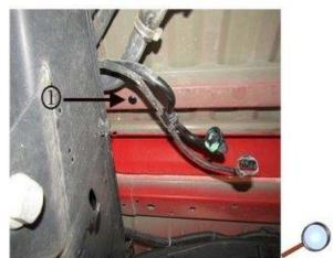
Before reinstalling the fuel tank to the vehicle, install one drain hole plug (1) to the open left side drain hole location shown above. Document ID: 4540463 Page 4 of 7
