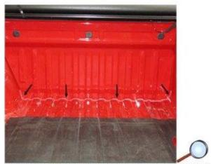
Ensure the complete front joint is sealed, and allow to dry per manufacturer's recommendation.
