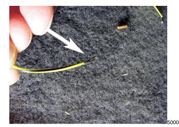
11. Fold the 13 mm (1/2 in) ends of exposed copper wires over each other.
