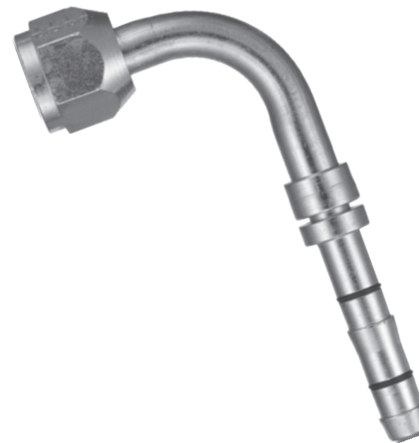
5/16 (-6) x 5/8-18 (-6) 90° Elbow Female O-Ring Short Pilot
